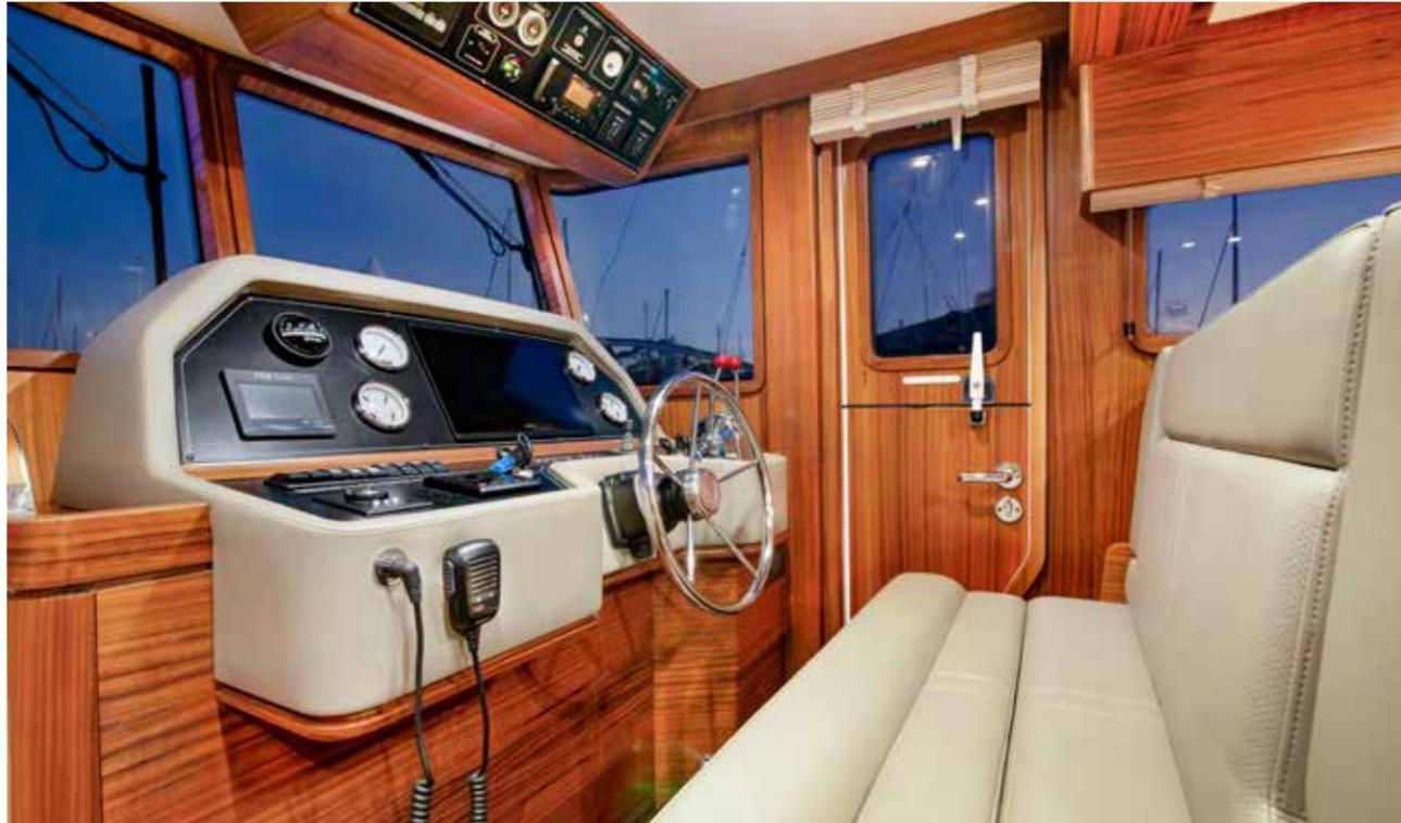
The hooded dash and reverse raked pilothouse windows prevent night reflections, and the dogging Dutch door provides easy deck access as well as a breeze.
